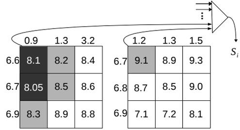
Figure 1: Cubes (grids) are fed to a priority queue (triangle) and generated hypotheses are iteratively popped from the queue and added to stack  $S_i$ . Lower scores are better. Scores of rules and hypotheses appear on the top and left side of the grids respectively. Shaded entries are hypotheses in the queue and black ones are popped from the queue and added to  $S_i$ .
