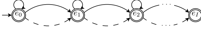
Figure 6.6: Error-correction model based on PFSMs for IMT given the sentence e_1^I : \mathcal{B}_{e_1^I} . The states of the PFSM are labelled with the words of the target sentence e_1^I .
