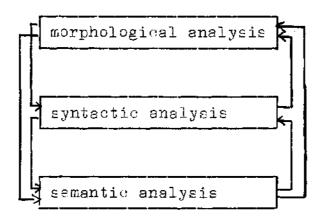
The scheme shows the "structure" of the program required for the analysis. The program begins with the morphological analysis of the word forms of a given text. In the case of homographic forms also syntactic and semantic relations are taken into consideration. As a result C.II. will be stored.
