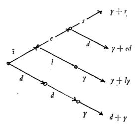
In this representation, if several rules begin in the same way, the similar parts are only represented once and if the similar initial parts of a set of rules are matched against a set of edges, this will be a partial test of all the rules in the set. In the computer, this can be represented as follows:
